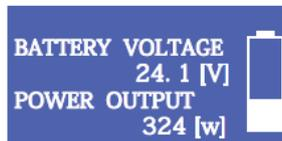
2. To display Power Status in voltage and watt, when using the battery.
