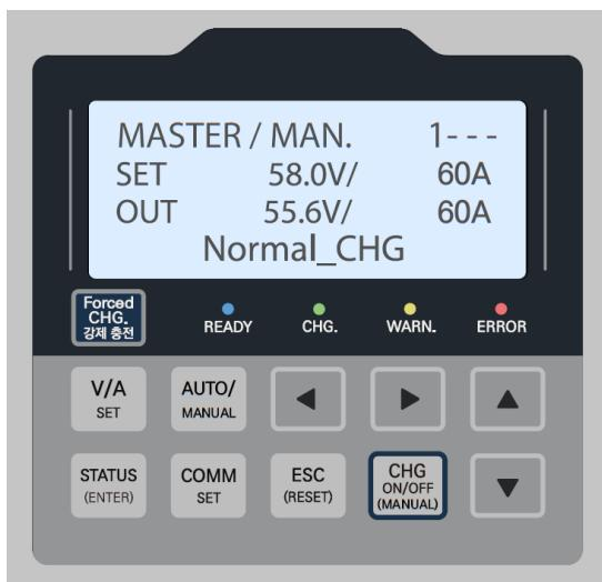
A. **[V/A SET] button** --> Max Charge Voltage, enter the maximum charge voltage.
