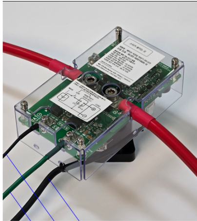
UI (User Interface)용 커넥터 전선 (-) from Battery (for control power) F.G. (Frame Ground)
